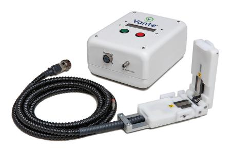
The TPE Sealer produces consistent, quality seals on most TPE tubing used in biopharmaceutical manufacturing. This sealer is easy to clean, portable and compact. One-button operation makes this sealer easy to use and validate. The unique remote thin wall sealing head clamps and hangs from tubing for convenient use with manifold systems. The Thin Wall Sealing Head seals thin wall (.062) tubing: .125 OD - .375 OD. Operates 100-240V, 50/60 Hz outlet (Compressed air required) CE marked.
